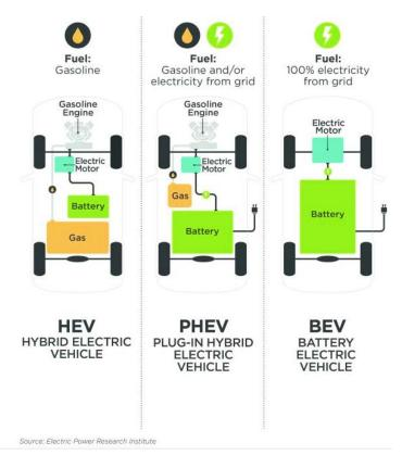
Figure 1: Schematic Showing Elements of a HEV, PHEV and BEV<sup>5</sup>
